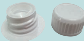
F&N product cap after removal of the tamper-proof ring
